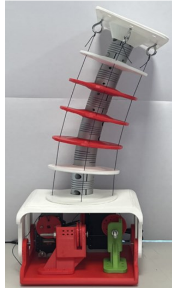
Fig. 7. Prototype of the vertebra-disk unit torso for a new LARMbot Humanoid, [23]
