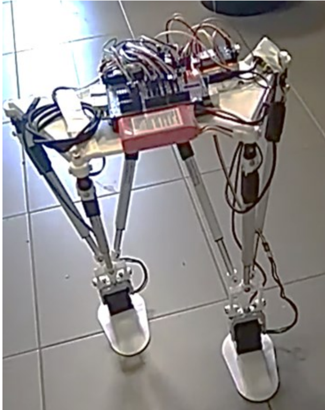
Fig. 6. Prototype modules for a new LARMbot Humanoid: a) leg with ankle assisted foot,[21]; b) arm with elbow actuated joint, [22]
