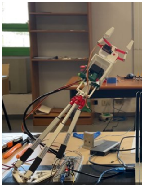
Fig. 7 A snapshot of a lab test of the manipulation capability of the tripod-based leg arm
